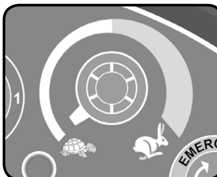
Set to slowest speed, depress accelerator and drive off the pallet using ramp provided.
